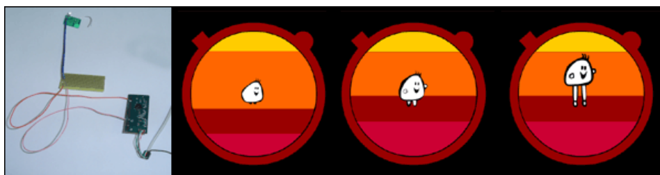
Figure 14: interface investigation: a Mascot in various growth stages. The color strips in the background indicate the communication levels of each of the group members A mobile phone radiation sensor was used to indicate calls and messages sent to the phone and controlled the changes in the interface.
