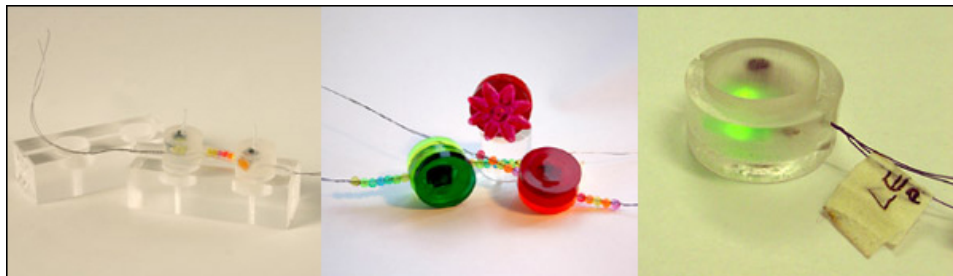
Figure 18: Silicone molds test, checking for component sizes, first working bead unit
